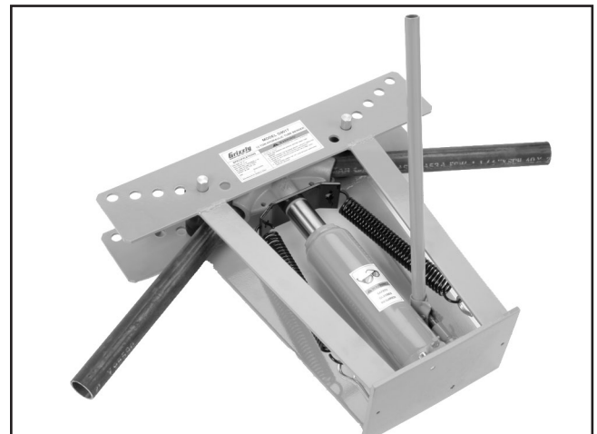
Figure 6. Rollers set close together for bending short pipes.
