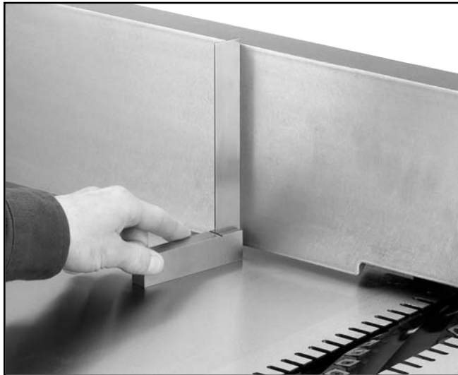
Figure 41. Use of square to align fence.
