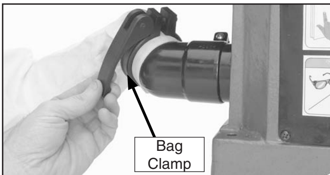
Figure 20. Attaching the dust collection bag.
