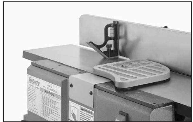
Figure 27. Checking the 90° stop.
