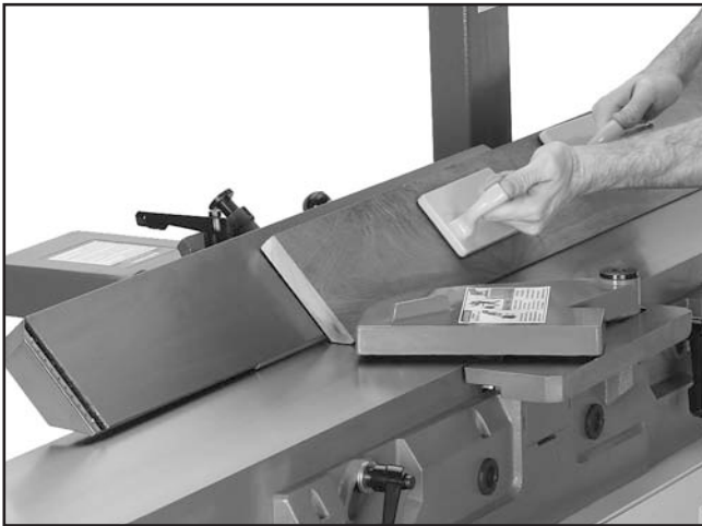
Figure 41. Example photo of a typical bevel cutting operation.
