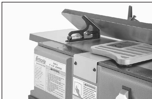
Figure 28. Checking the inward 45° stop.
