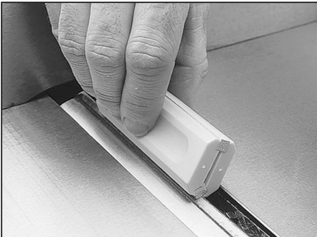
Figure 42. G3631 Jointer/Planer Knife Hone.
