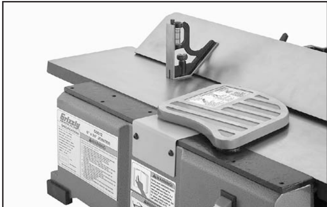
Figure 30. Checking the outward 45° stop.
