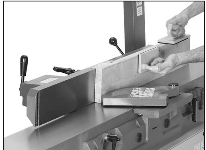
Figure 37. Example photo of a typical jointing operation.
