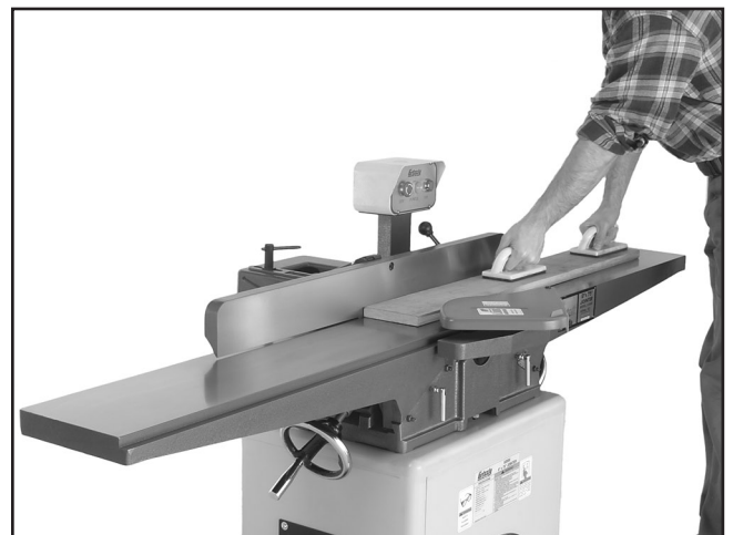
Figure 26. Typical surface planing operation.
