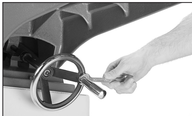
Figure 12. Securing the handwheel handle.
