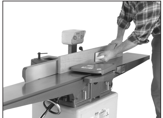
Figure 28. Typical edge jointing operation.
