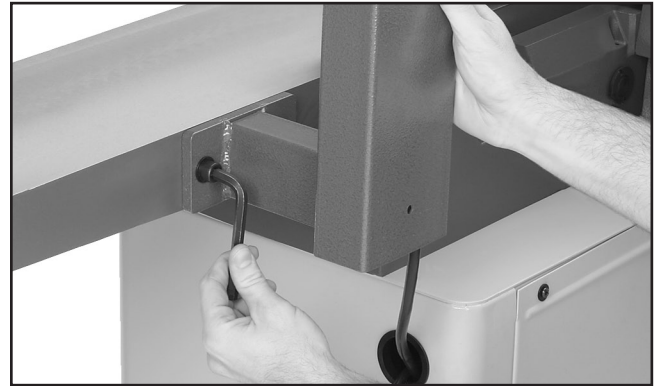
Figure 15. Attaching pedestal switch to stand.
