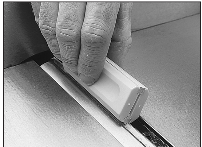
Figure 37. G3631 Jointer/Planer Knife Hone.
