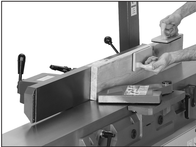
Figure 30. Typical edge jointing operation.
