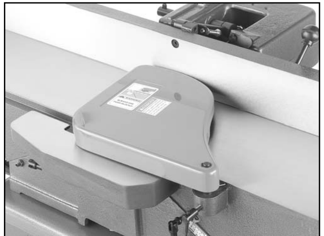
Figure 38. Cutterhead guard properly positioned over cutterhead and against fence.
