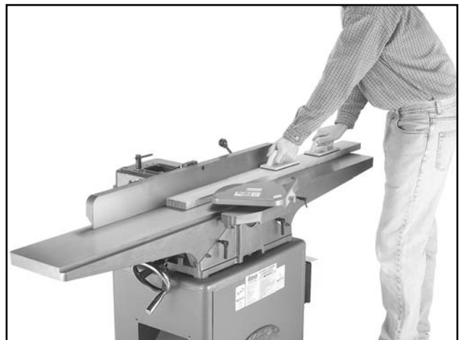
Figure 45. Surface planing the face of a workpiece.
