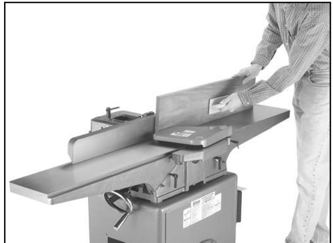
Figure 47. Edge jointing a workpiece.
