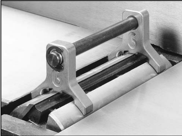
Figure 53. Jig placement on cutterhead.
