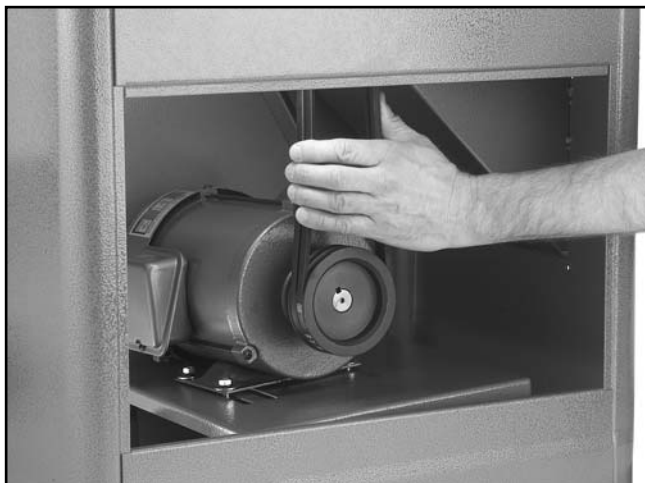
Figure 58. Checking V-belt tension.
