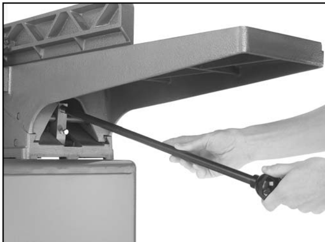
Figure 25. Installing table lever into adjustment block.
