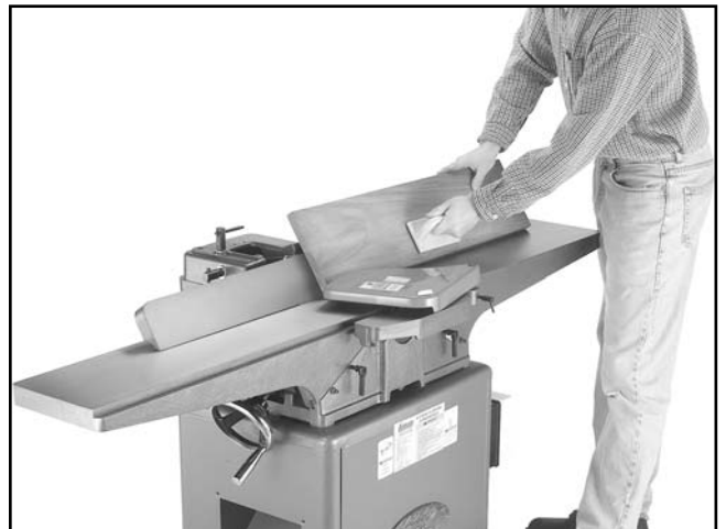
Figure 49. Bevel cutting with the fence at 45°.
