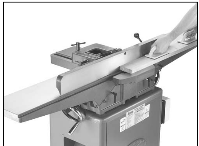
Figure 51. Rabbet cutting a workpiece.
