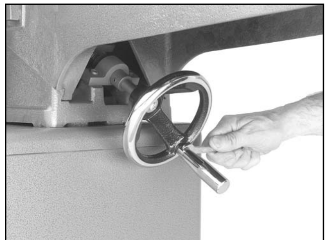
Figure 24. Installing handle into handwheel.
