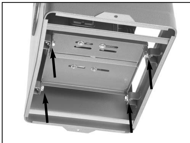
Figure 60. Motor adjustment bolts (shown underneath stand for clarity).
