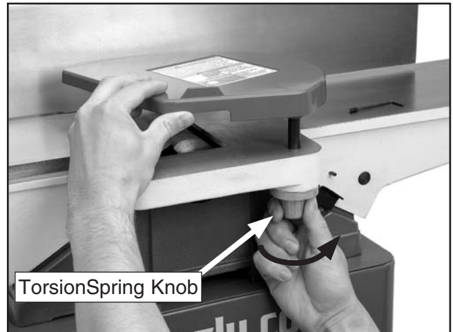
Figure 18. Setting torsion spring knob.
