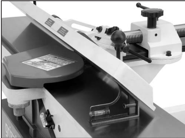
Figure 58. Adjusting fence 45° inward.
