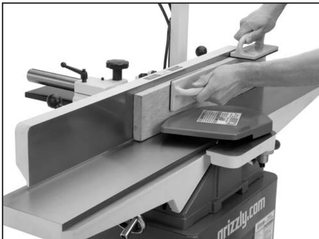
Figure 35. Typical edge jointing operation.
