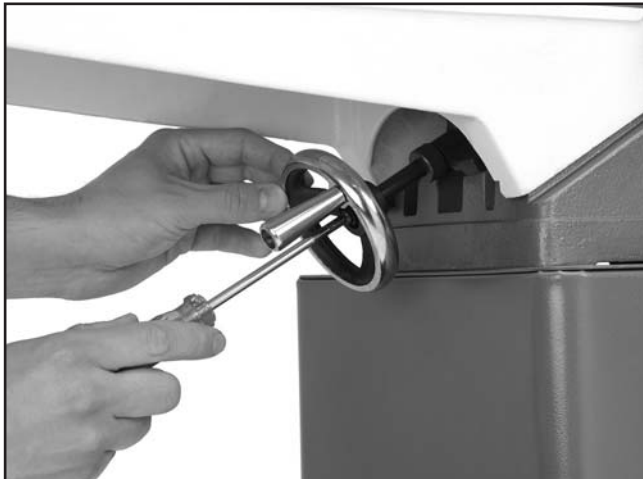
Figure 23. Securing the handwheel.
