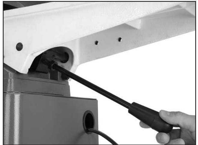
Figure 24. Installing infeed table lever.
