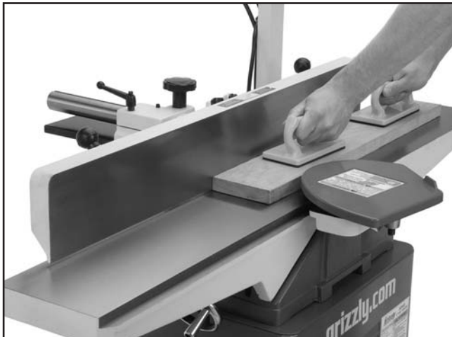
Figure 33. Typical surface planing operation.
