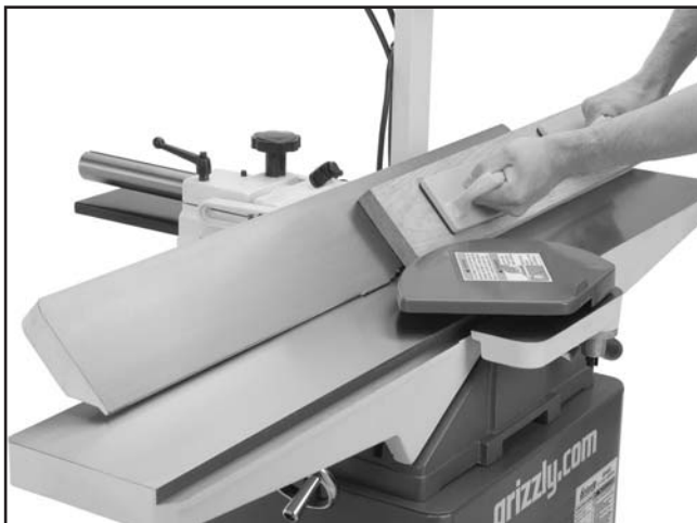
Figure 37. Typical bevel cutting operation.
