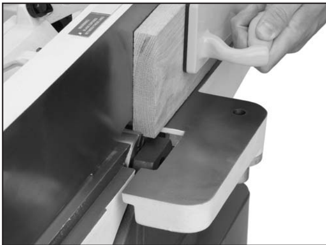
Figure 39. Typical rabbet cutting operation.
