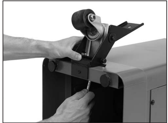
Figure 6. Installing locking foot pedal.
