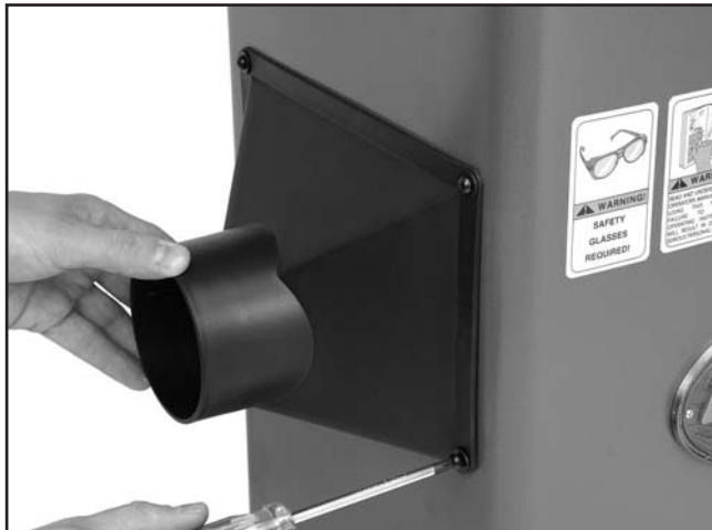
Figure 20. Dust port installation.
