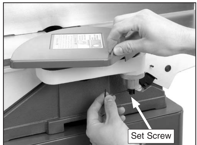
Figure 19. Reinstalling set screw.
