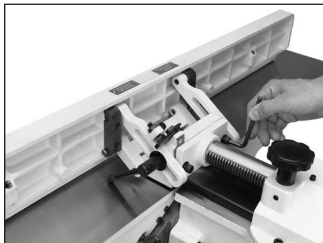
Figure 15. Installing fence assembly.
