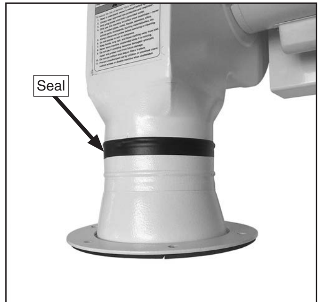
Figure 4. Electrical tape wrapped around seam between collection flange and outlet.
