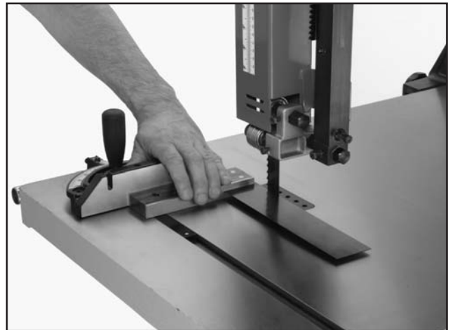
Figure 17. Squaring miter gauge to blade.
