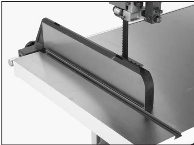
Figure 18. Fence square with miter slot.
