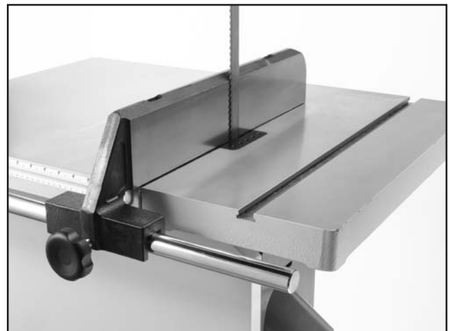
Figure 19. Fence flush with blade.
