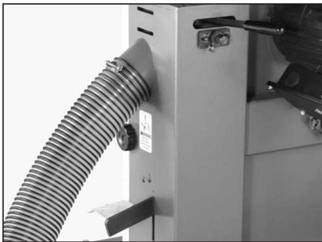
Figure 20. Dust hose attached to dust port.
