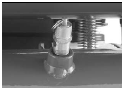
Figure 8. Safety drain valve.
