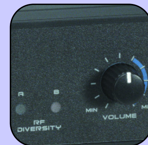
RECEIVERS BODY HAS ROTARY VOLUME CONTROL & CH/RF LEDs
