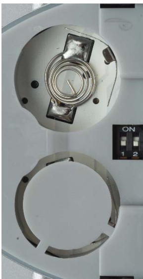
Left: Picture of the opened rear battery compartment of the RMT4-IR remote showing the exposed DIP Switch bank between the battery chambers.
