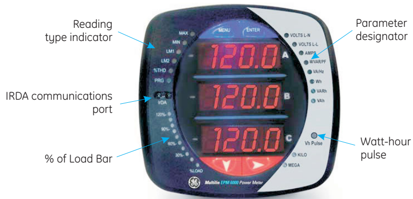
FIGURE 4-1: EPM 6000 Faceplate Elements
