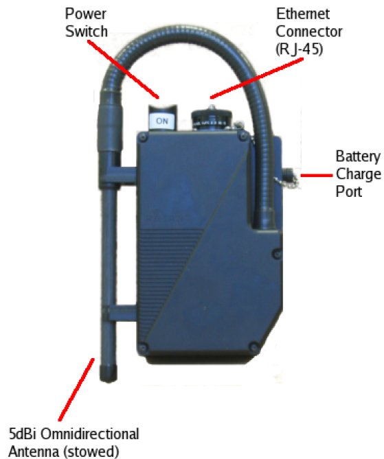
Figure 3-2. BreadCrumb WE - External Connectors
