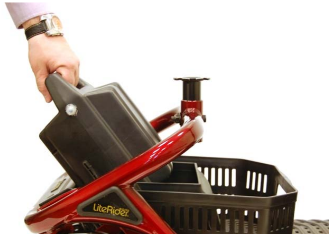
Figure 21. Battery Pack Installation
