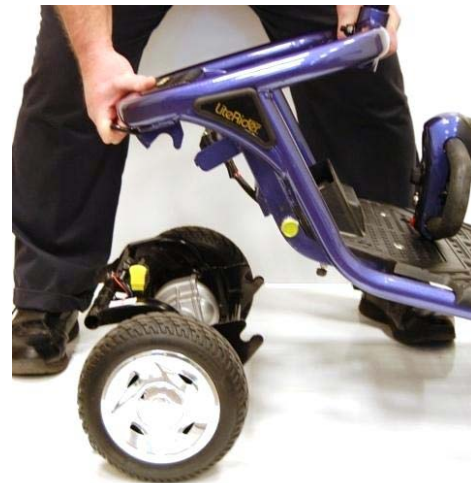
Figure 18. Lifting the Frame
