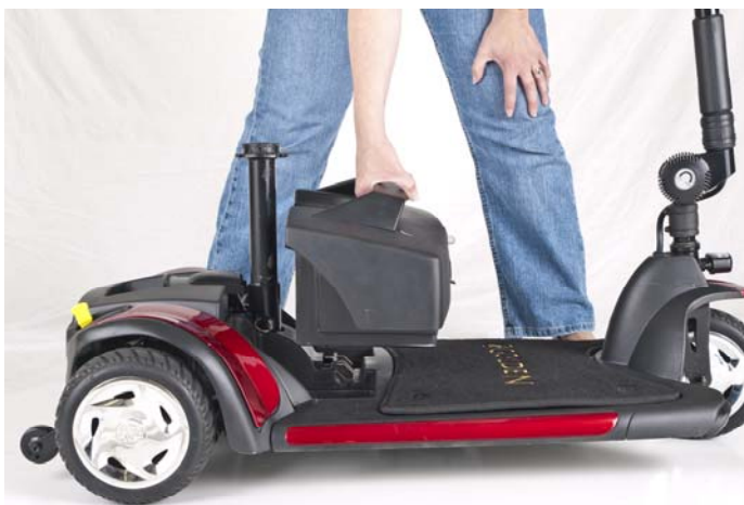
Figure 22. Battery Pack Installation
