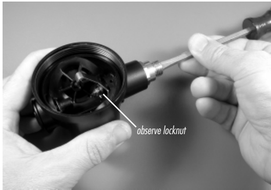
Fig. 18 – Orifice Preliminary Setting
