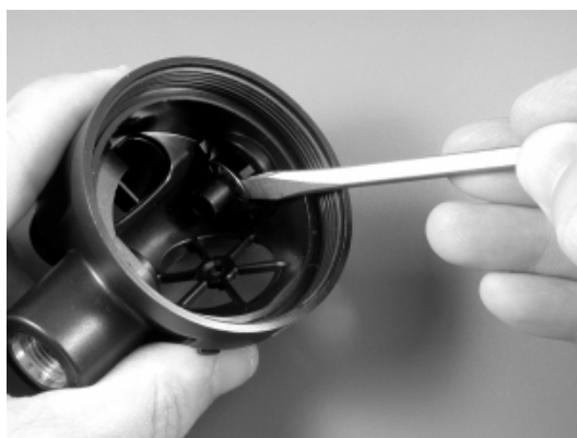
Fig. 12 – Case Plug Removal
