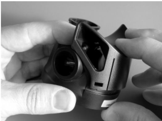
Fig. 14 – Exhaust Tee Installation
