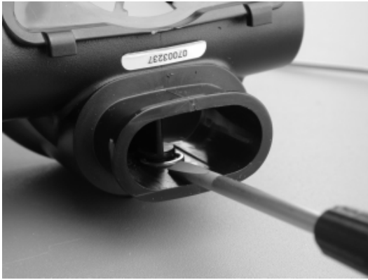
Fig. 13 – Atlas Retaining Ring Installation
