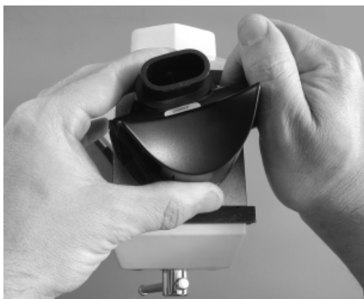
Fig. 6 – Cover Ring Removal
