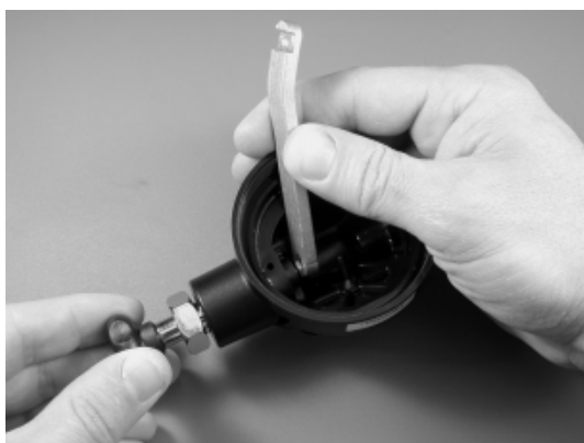
Fig. 8 – Disassembly of Poppet
