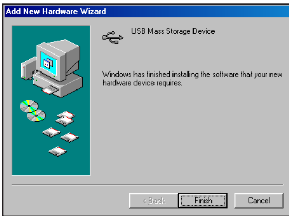
Figure 14. Completing Driver Installation
