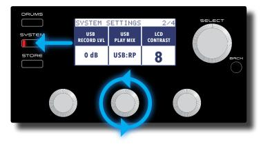
level. As you adjust the control clockwise, you can vary the RP signal level in relation to the USB playback level. This parameter is only available when a USB connection has been made to the RP.
