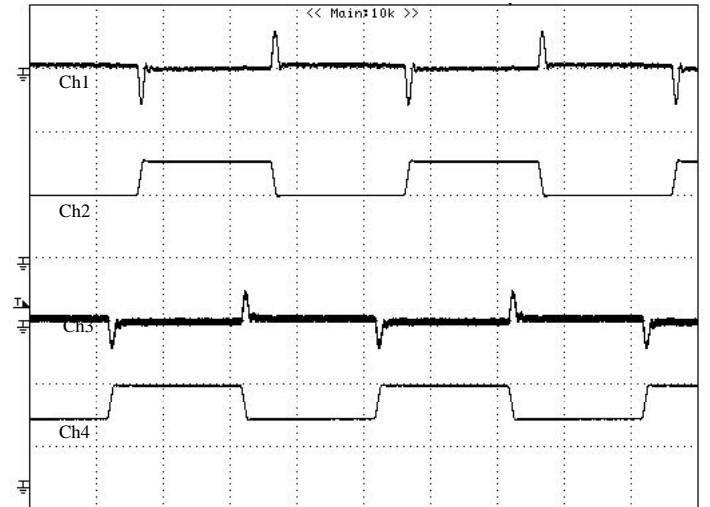
Figure 12: Output voltage response to step-change in load current I_{out2} and I_{out1} (75%-50%-75% of I_o , max; di/dt = 0.1A/\mu s ). Load cap: 10\mu F , tantalum capacitor and 1\mu F ceramic capacitor. Ch1= V_{out2} (100mV/div), Ch2= I_{out2} (7.5A/div), Ch3= V_{out1} (100mV/div), Ch4= I_{out1} (7.5A/div) Scope measurement should be made using a BNC cable (length shorter than 20 inches). Position the load between 51 mm to 76 mm (2 inches to 3 inches) from the module.
