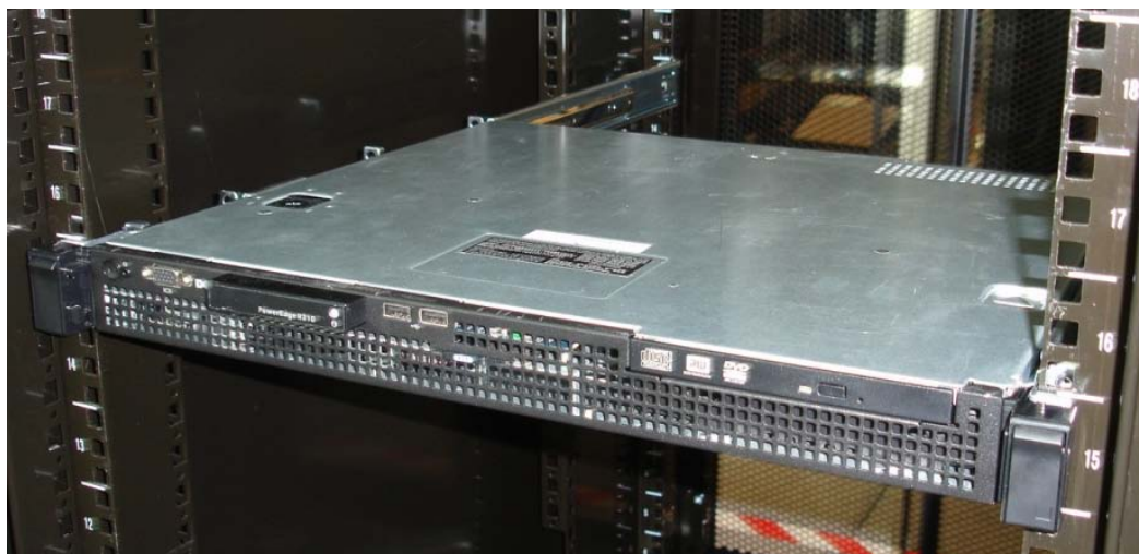
Figure 8. R210 Mounted In Four-Post Square-Hole Rack
