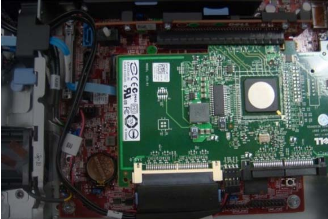
Figure 14. SAS 6/iR Adapter Card Installed
