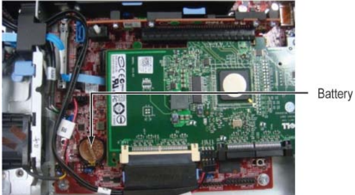
Figure 12. Battery on Motherboard
