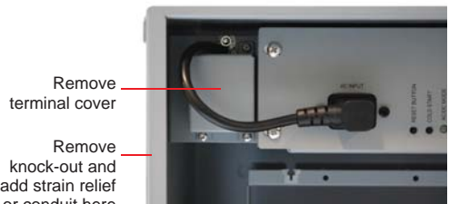
Figure 14: AC Wiring (i)
