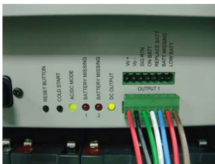
Figure 16: LED's and ONT Alarm Connections
