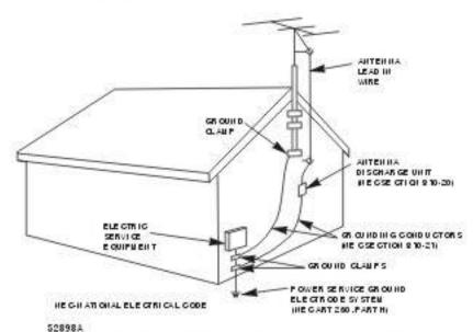
EXAMPLE OF ANTENNA GROUNDING AS PER ANTIONAL ELECTRICAL CODE
