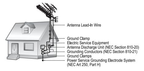
sure the antenna system is grounded so as to provide some protection against voltage surges and built-up static charges. Article 810 of the National Electrical Code, ANS/NFPA 70 provides information with regard to proper grounding of the mast and supporting structure, grounding of the lead-in wire to an antenna-discharge unit,
