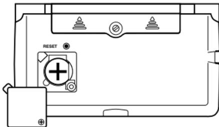
3. Insert a thin, pointed object into (A) and remove the old battery.
