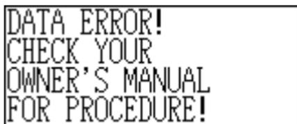
Appearance of the data error message indicates that you must perform the all-reset procedure to correct the problem. Start out with the procedure under "To start the all-reset operation" on page 11, and continue with the procedure under "When to press Y for "yes"" on page 11.
