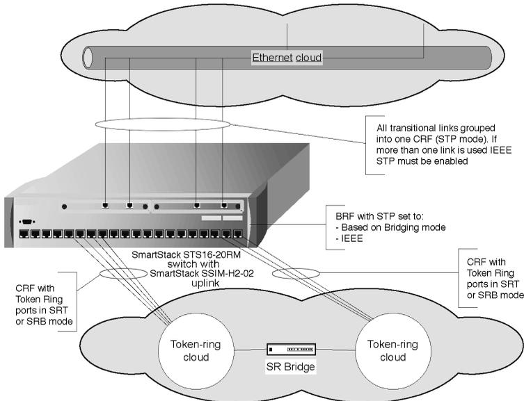
**Figure 5. Ethernet CRF in SRB Bridging Mode**
