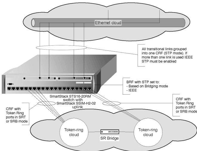
**Figure 4. Ethernet CRF in SRT Bridging Mode**
