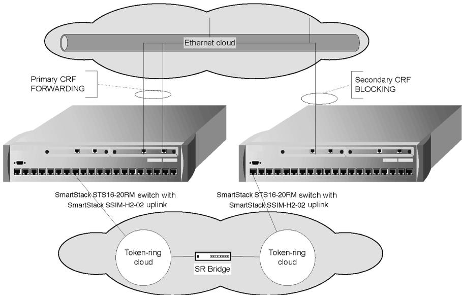
**Figure 9. Redundant Connections to Fast Ethernet Network**
