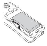
3 Install the battery cover by sliding it onto the back of the handset.
