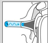
Braun ThermoScan measures the infrared heat generated by the eardrum and surrounding tissue. To help ensure accuracy, the thermometer «scans» by taking 8 measurements in just one second and displaying the highest temperature.
