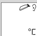
6. If no button is pressed or no new probe cover is attached within 30 seconds, the thermometer will turn off automatically.
