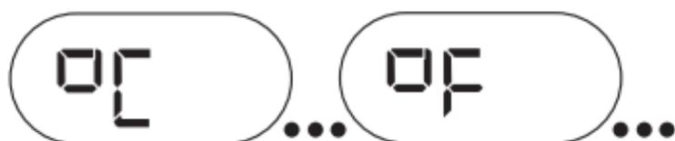
Release the «start» button when «°F» is shown. There will be a short beep to confirm the new setting, the thermometer then turns off automatically.
