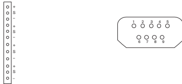
LTC 8569 Series: 8 12-Pin Connectors LTC 8569/60 Series and LTC 8571/60 Series: 2 D-Connect LTC 8571 Series: 16 12-Pin Connectors LTC 8570/60 Series and LTC 8572/60 Series: 4 D-Connect
