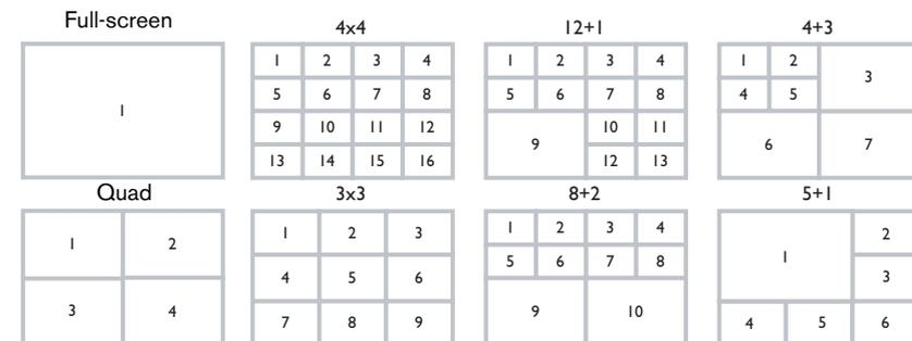
The quad mode can have 4 different quad screens that can be shown in sequence to display 16 camera pictures.
