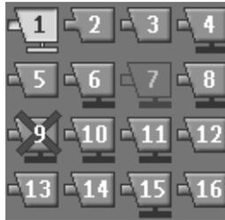
The camera icons show the number of the camera connection. The status and type of camera is indicated by the type of icon used.
