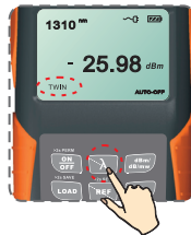
Figure 4-6. Press and hold to activate auto-wavelength recognition.
