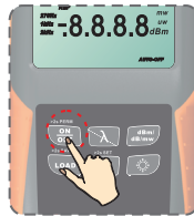
Figure 4-4. Powering on the power meter.
