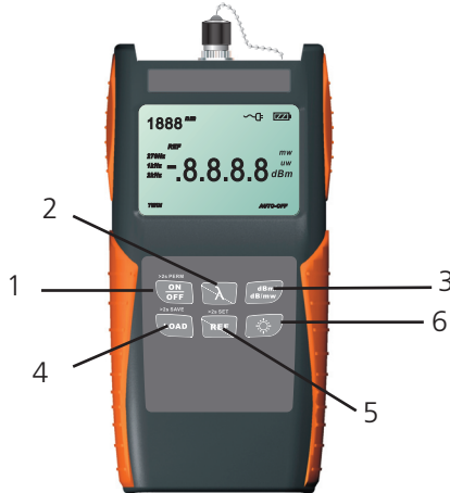
Figure 4-1. Keypad functions: Number 1 through 6.
