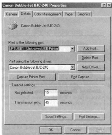
4. If the USB Parallel Printer Adapter is not plugged in, you will see the message under the "Print to the following port" box in Figure 3. Plug the Belkin USB Parallel Printer Adapter into the printer as show in Step 4 of New Installation.
