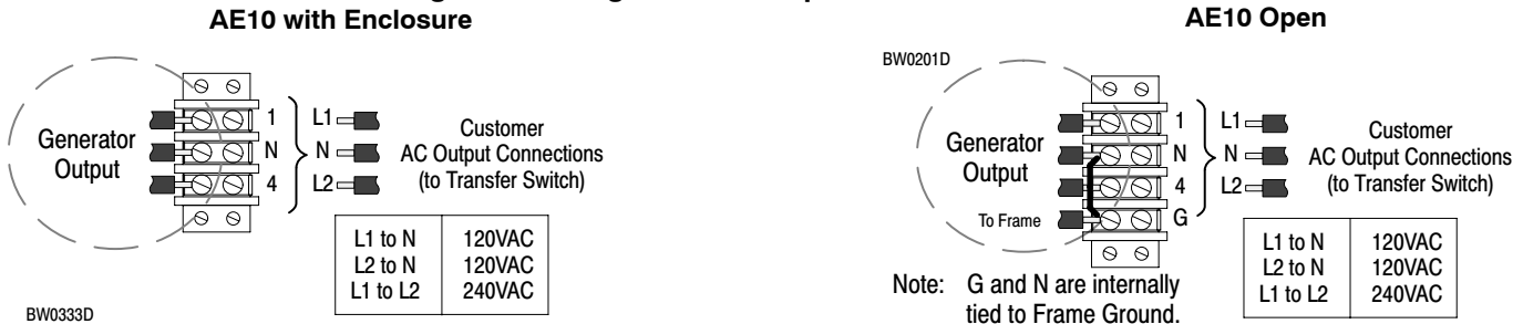
Figure 3-5 Single Phase Output Power Connections
