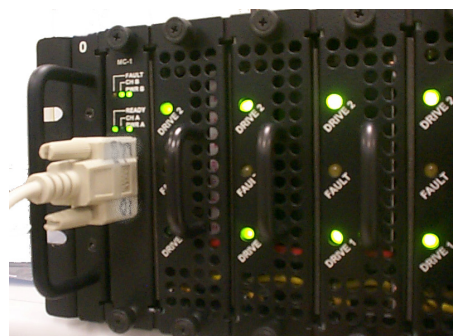
Exhibit 10-1: The management card may be accessed via a serial port DB-9 connector or an optional Ethernet connection.
