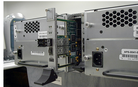
Exhibit 10-3: The Fibre Channel or SCSI Host Interface Card may be replaced by shutting power down, removing any cable attached to the port, removing the GBIC or SFP according to manufacturer's instructions, loosening the screws at the top and bottom of the card, then carefully pulling out the unit.
