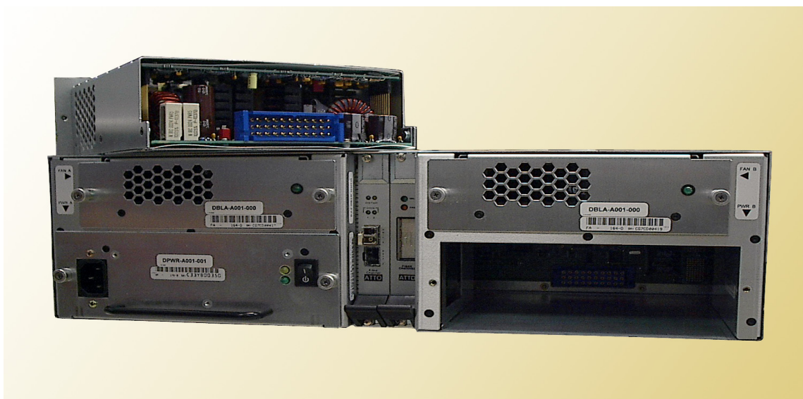
Exhibit 10-4: A power supply pulled out from a rackmount Diamond Storage Array: do not leave an empty opening while the Diamond Storage Array is operating. Access the blower assembly and the power supply by loosening the screws on either side of the component, then pulling out the part. If a blower or power supply stops working, keep it in place until another component is installed. (Note: host interface configuration pictured is not supported)
