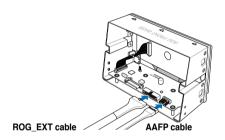
Insert the other end of the ROG\_EXT cable and the AAFP cable through the two empty 5.25-inch drive trays.
