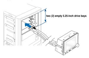
Align and place the ROG Front Base with its connected cable to the two (2) empty 5.25-inch drive bays.
