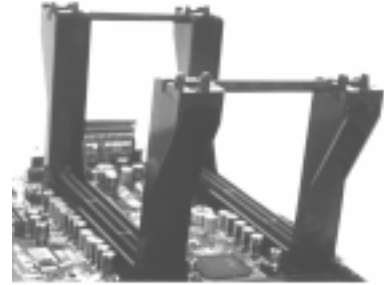
Both retention mechanisms with both brace bars installed
