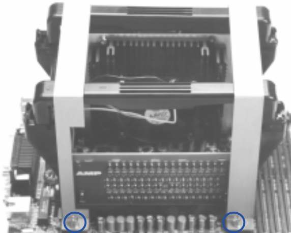
Retention mechansim fram around single processor configuration with terminator.
