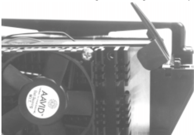
The processor raised out of the slot 2 connector by the reverse force of the lifters as they are pryed to a vertical position.
