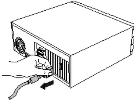
**Note:** If you are disconnecting a peripheral from the computer or are removing a component from the system board, wait 10 - 20 seconds after disconnecting the computer from the electrical outlet before disconnecting the peripheral or removing the component to avoid possible damage to the system board. To verify that all power has been removed from the system, make sure that the standby power light-emitting diode (LED) on the system board has gone out.
