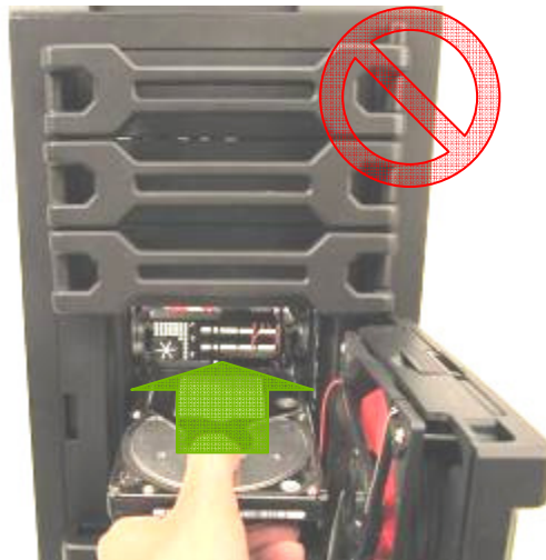
Installing a 3.5" internal device
