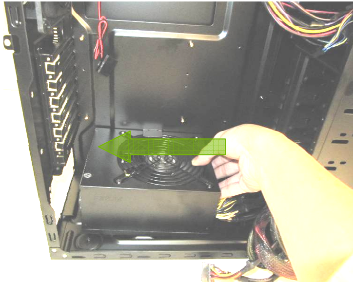
PSU resting on the standard PSU mount.
