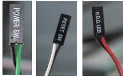
Front Panel switch leads
