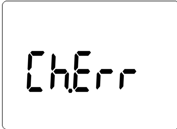
Figure 6-3 Charge terminal alert
