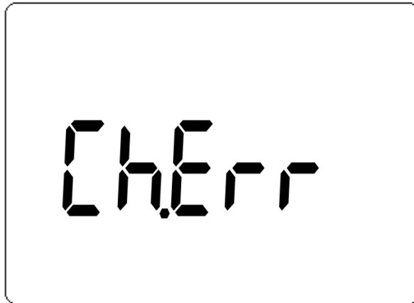
Figure 2-17 Charge terminal alert
