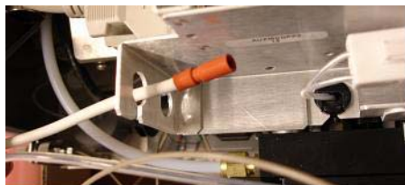
Figure 8 Connecting the APCI HV to the chassis.
