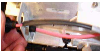
Figure 9 Connecting the HV PCA to the chassis.
