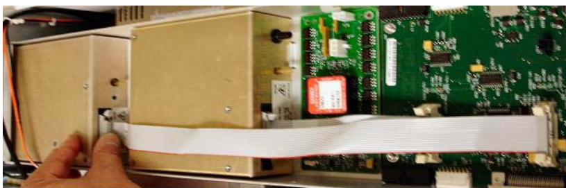
Figure 7 Connecting the APCI HV power supply to the valve PCA.
