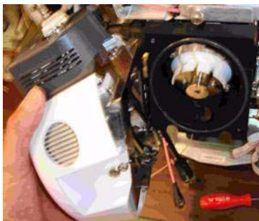
Figure 10 Installing the multimode source (left) and connecting all connectors.
