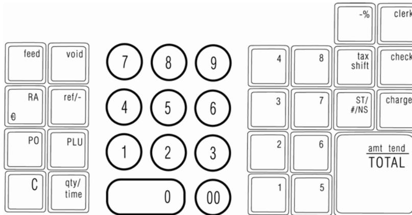
1. **[ Feed ] - Paper Feed Key** - Advances the paper tape with no effect on register entries.
