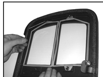
Fig. 7 Fitting door glass
