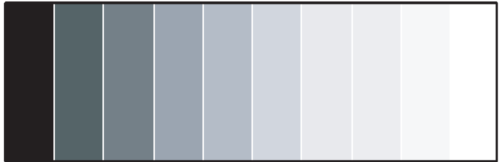
Figure 4-3. Typical Gray Bar Pattern for Adjusting Contrast
