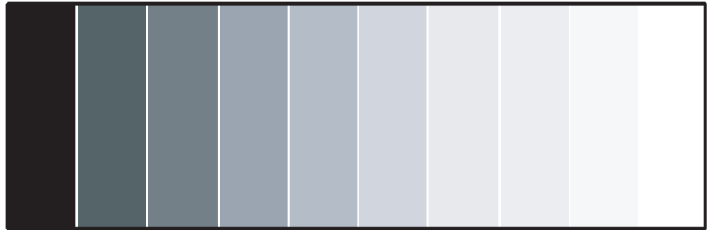
Figure 4-3. Typical Gray Bar Pattern for Adjusting Contrast
