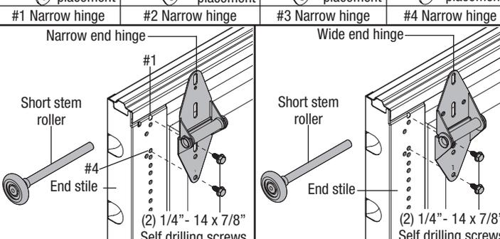
(A) NARROW END HINGE INSTALLATION (B OR C) WIDE END HINGE INSTALLATION
