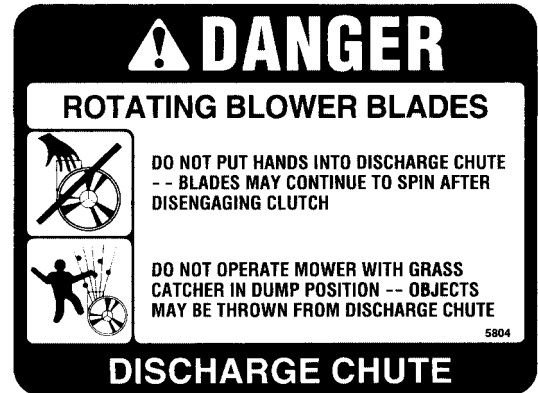
Adjacent to Blower Discharge Chute through Body (5804)
