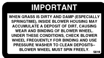
Top of Blower Housing (5819)
