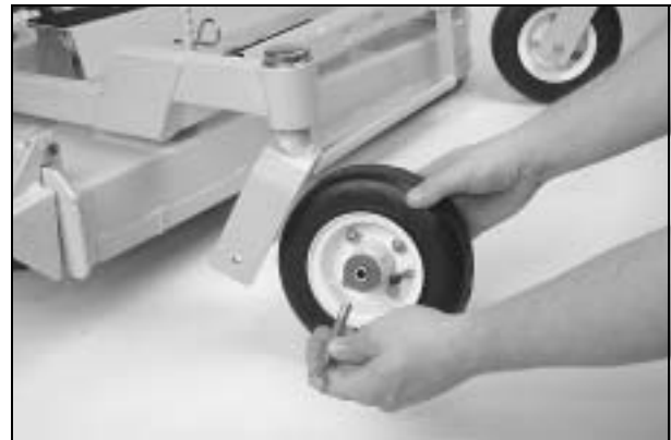
Deck Caster Wheel Installation
