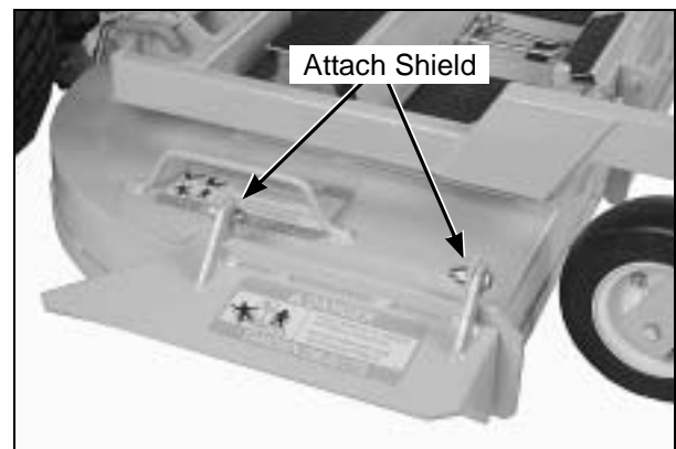
Deck Discharge Shield Installation
