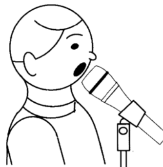
DISTANCE FROM MICROPHONE AFFECTS PERFORMANCE FIGURE 1
