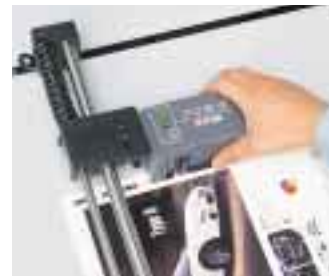
RYOBI PDS-E printing density control system (option)
